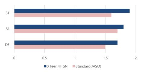
STI -Stop Time Index: how quickly the clutch engages
